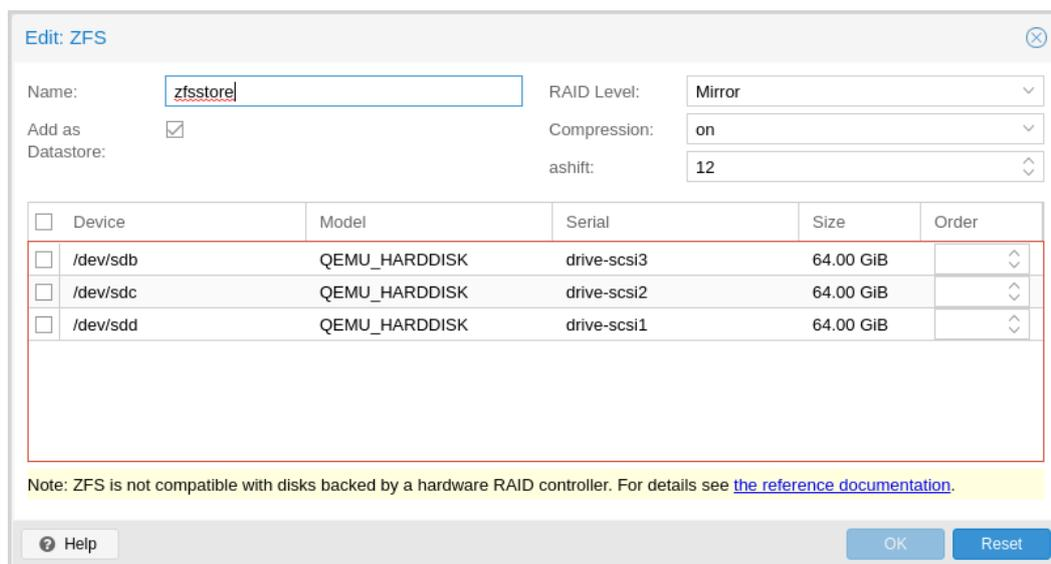
You can also create a `zpool` with various raid levels from **Administration -> Disks -> Zpool** in the web interface, or by using `zpool create`. The command below creates a mirrored `zpool` using two disks (`sdb` & `sdc`) and mounts it on the root directory (default):
