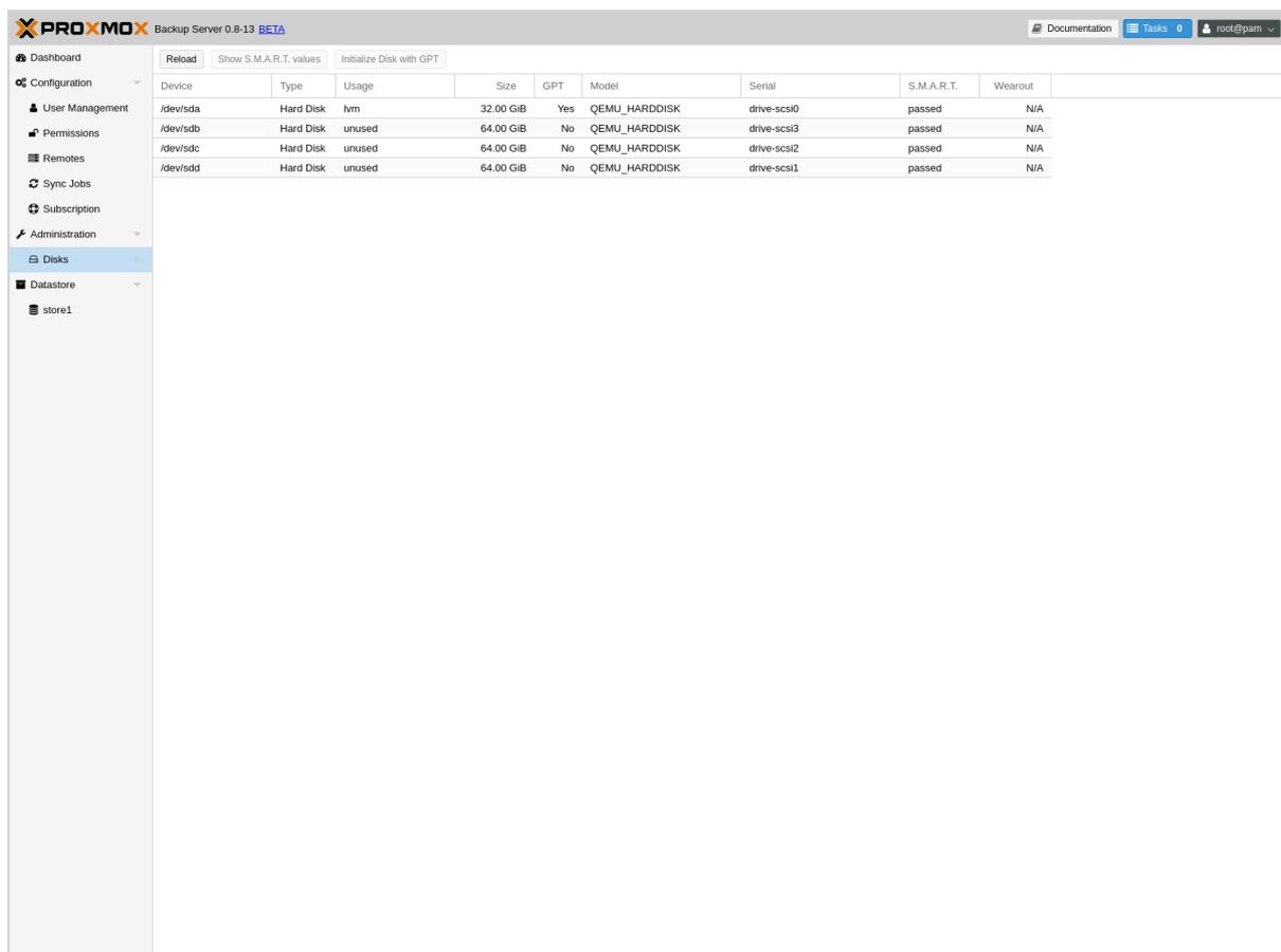
Proxmox Backup Server comes with a set of disk utilities, which are accessed using the `disk` subcommand. This subcommand allows you to initialize disks, create various filesystems, and get information about the disks.
