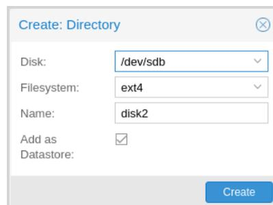
You can create an ext4 or xfs filesystem on a disk using `fs create`, or by navigating to **Administration -> Disks -> Directory** in the web interface and creating one from there. The following command creates an ext4 filesystem and passes the `--add-datastore` parameter, in order to automatically create a datastore on the disk (in this case `sdd`). This will create a datastore at the location `/mnt/datastore/store1`:
